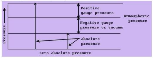
Diagram showing absolute pressure, vacuum and gauge
